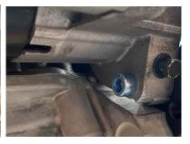
4) Place the factory VR/VQ automatic transmission flexplate onto the engine being sure to align the indicator pin correctly on the crankshaft. **DO NOT INSTALL** the VR/VQ torque plate (this is the thin metal plate that has 8 holes and was originally sandwiched between the heads of the flexplate bolts and the flexplate.
