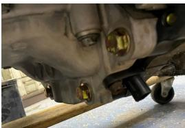
!!WARNING!! - If adapter plate does not seat fully onto dowels, use a hammer and a block of wood to tap adapter down until it is flush with the engine block, DO NOT use the bolts to pull the plate down, as damage to the plate can result!
