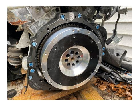
6) Install the RB Transmission to Engine alignment dowels in the adapter plate (not included). These are factory Nissan parts, and the part numbers are given in the beginning of this document. The larger dowel will be a tight fit and must be driven in with a hammer. Be sure not to over-drive this dowel as it can be pushed out the back and into the starter.
