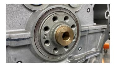
3) Install the adapter plate to the engine using two OEM VQ Engine to Transmission alignment dowels (not included) and supplied mounting hardware. Qty. 2 M10x1.5 25mm long socket head bolts will hold the adapter in place on the engine as shown below.
