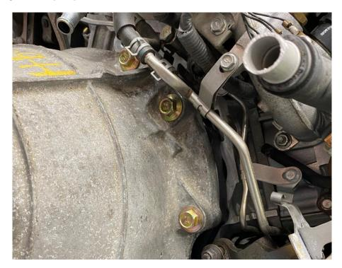
12) Along the bottom of the engine, 3 of the supplied M10x1.50 60mm long bolts will attach the engine to the transmission by passing through the three holes that were drilled out earlier in the instructions. 1 of the M10x1.50 60mm long bolts will pass through the transmission into the adapter plate below the starter, and the last will be used on the RH side of the transmission holding it to the adapter plate.
