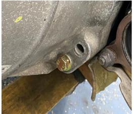
13) Lastly, The M10x1.50 35mm long flange head bolt and M8x1.25 35mm long socket head bolt will be used to attach the oil pan and transmission to the adapter plate, respectively. The M10 flange head bolt will install through the last hole in the oil pan, and the M8 bolt will pass through the threaded hole on the bottom RH side of the bellhousing.
