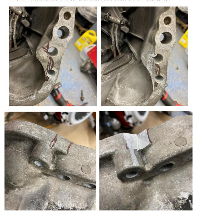
8) Test fit the transmission to the engine to ensure there is sufficient clearance for the starter snout inside the bellhousing and for the starter mounting bolt.
