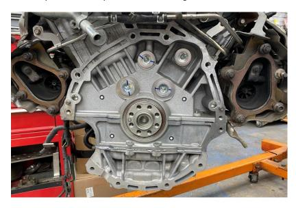
2) Install the custom pilot bushing to the VR38DETT Crankshaft
