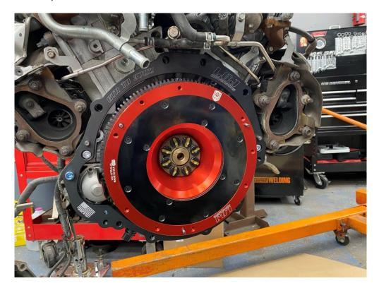
10) Install the 350Z/370Z clutch onto the flywheel following the manufacturers recommended practices.
