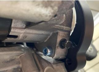
6) Install two additional OEM 370Z engine to transmission alignment dowels into the adapter plate.
