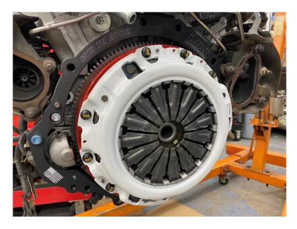
11) Reinstall the transmission to the engine. Along the top of the engine, use the 4 supplied M12x1.75 80mm long bolts to attach the transmission to the engine block. These bolts will pass through the adapter plate.
