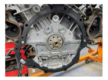
!!WARNING!! - If adapter plate does not seat fully onto dowels, use a hammer and a block of wood to tap adapter down until it is flush with the engine block, DO NOT use the bolts to pull the plate down, as damage to the plate will result!
