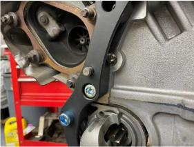
7) There is a boss above the starter pocket on the Z transmission that will need to be removed to allow the GTR starter to fit properly. Using an appropriate cutoff tool, modify the bellhousing as shown. A second notch will need to be cut to clear the head of the M10 starter bolt.
