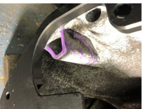
3) Remove the adapter plate and use grinder to remove the casting bosses to ensure your starter snout has sufficient clearance.
