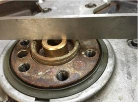
2) Before installing the adapter plate onto the engine, you will need to place the adapter onto the transmission to identify the location where a casting rib needs to be removed from the inside of the bellhousing. Mark the rib as shown in the picture on the right.
