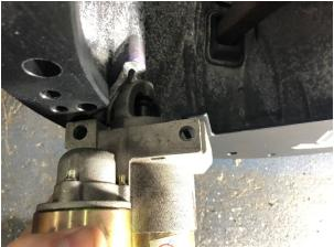
4) Install the LOJ Conversions Transmission Adapter Plate onto your Engine. Use the Seven M10x1.5 30mm Low-Profile Socket Head Cap Screws. If your engine did not have alignment dowel pins, install them before installing the adapter plate! Additionally, if you are using an aftermarket oil pan that does not utilize the lower two bolt, leave them uninstalled.
