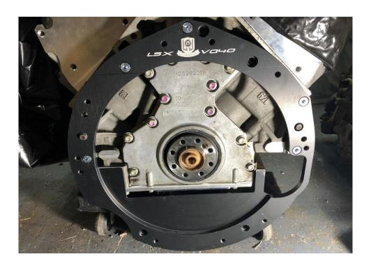
5) Now install your flywheel onto the engine. Apply Loctite 242 thread locker (optional, not included) to the thread of the flywheel bolts and install according to factory specs.
