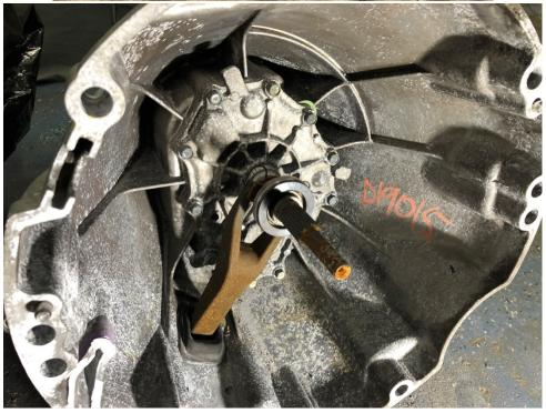
8) You are now ready to install your transmission onto the engine. Using the Ten M10x1.5 hex bolts and M10 flat washers, attach the transmission to the engine. WARNING: The washers MUST be used, without the washers the bolts will protrude past the back of the adapter plate and damage to the engine/adapter will result!
