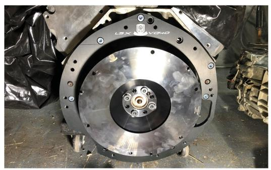
6) Now install your clutch onto the flywheel according to the manufacturer's instructions. LOJ recommends using Loctite Blue on the pressure plate bolts.
