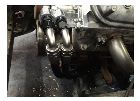
4) Your installation is complete. Start your engine and check for leaks. Tighten any connections if necessary.
