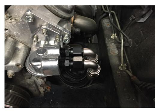
2) As seen in the images below, attach the 120 degree angle ends of the oil hoses to the oil pan fittings. The hoses should point up and forward and the hoses should be routed underneath the drivers side motor mount.
