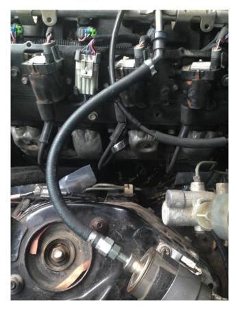
6) Your installation is complete. Pressurize the fuel system by cycling the ignition key and check for leaks.
