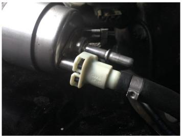
4) Install the Filter Return Fuel Line (Part "B") onto the <u>FRONT</u> hard line on the 300ZX framerail. The RETURN hose has the SMALLER quick disconnect fitting. Use the supplied clamp to fasten the line at the framerail, then route the hose along with the feed line up to the filter.
