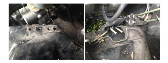
2) First, install the new filter/regulator (Part "D") onto the driver's side shock tower using the forward-most mount hole and one of the original M6x1.0 fasteners.
