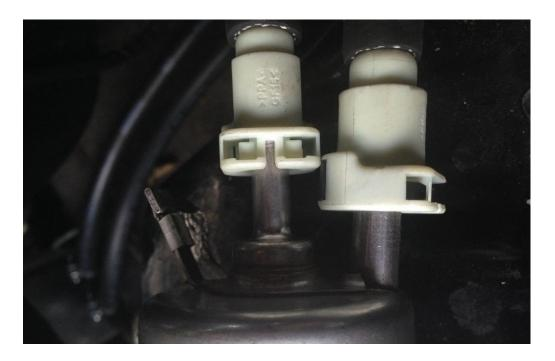
5) Now connect the filter/regulator to the fuel rail using the Filter to Rail Fuel Line (Part "C").
