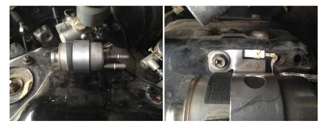
3) Install the Filter Feed Fuel Line (Part "A") onto the <u>REAR</u> hard line on the 300ZX framerail. You can identify the FEED hose from the RETURN hose, as the quick disconnect fitting on the FEED hose is LARGER than the return hose. Use the supplied clamp to fasten the line at the framerail, then route the hose under the brake master cylinder and up to the filter. See images below.
