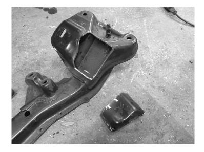
4) This piece can be trimmed and flipped over, then welded back into the same location it was cut out of.
