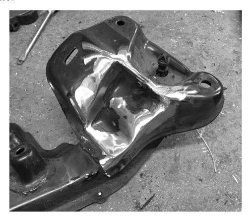
5) This will gain the required clearance to clear the bottom of the compressor when installed.
