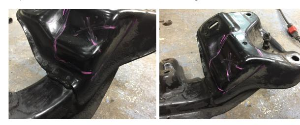
3) Cut this section out of the subframe, but SAVE the piece you removed!
