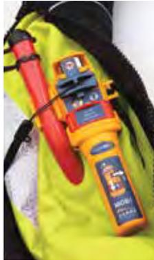
The RescueMe MOB1 is compatible with most inflatable lifejackets, simply clipping onto the oral inflation tube and activated by a wrap-around pull lanyard that triggers the arming cover and releases the antenna as soon as your lifejacket inflates, sending the first alert within 15 seconds.
