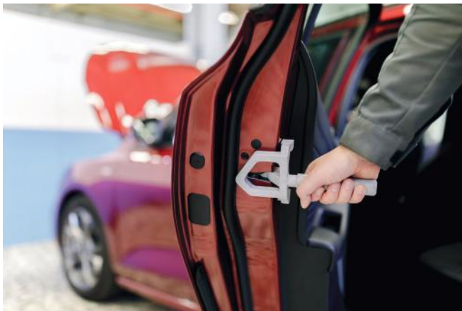
Ford saved costs and time by 3D printing tools and jigs for the new Focus
