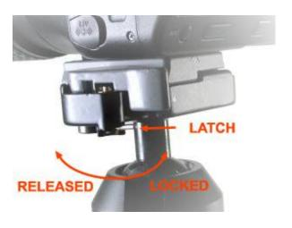
Plate is released by rotating QUICK RELEASE LEVER into hold open position. Plate attaches to camera with provided universal threaded screw mount and then snaps into position on tripod. QUICK RELEASE LEVER then closes and can be locked with QUICK RELEASE LATCH.
