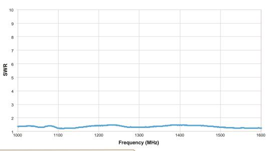
IRMS216 Rack Mount Splitter SWR vs Frequency
