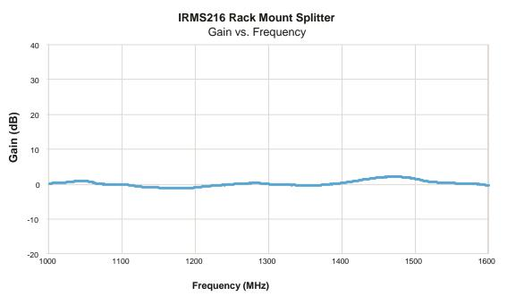
Figure 2-1. IRMS216 Splitter: Gain vs. Frequency
