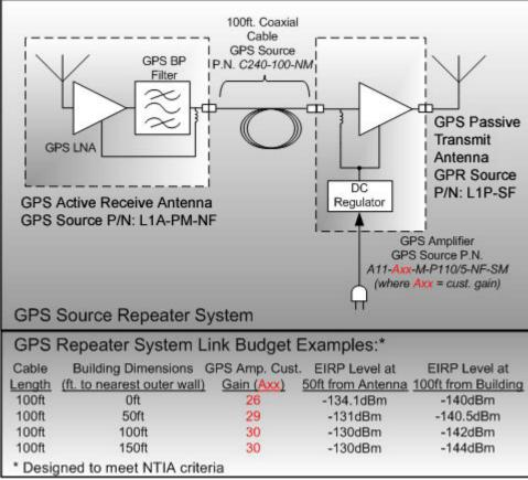
Figure 1. GPS Source typical Repeater System
