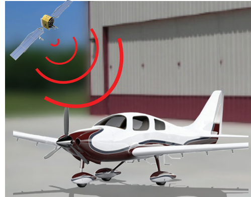
Aircraft Towed Outside of Hangar to Receive GPS Signal for MRO
