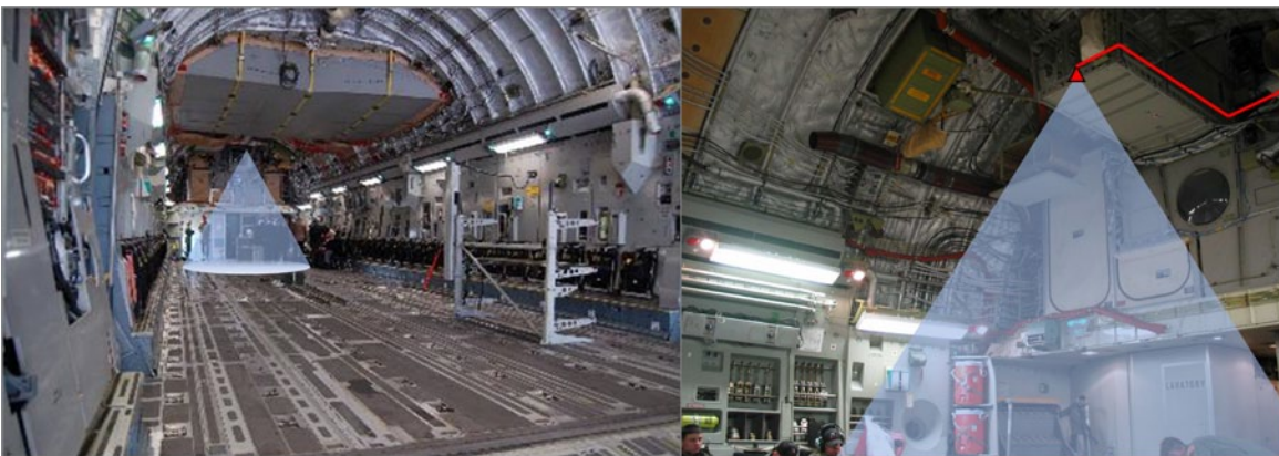
Figure 7. GPS Retransmission System Installed to USAF C-17 to Meet MFF Requirements
