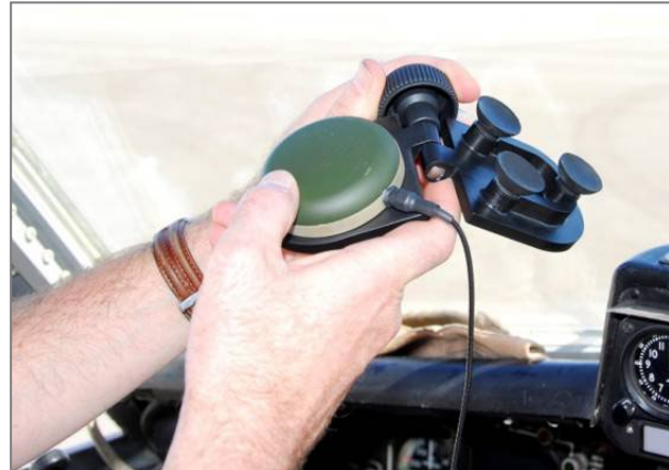
Figure 4. Suction Cup Mounted Active Antenna for Easy Retransmission System Installation
