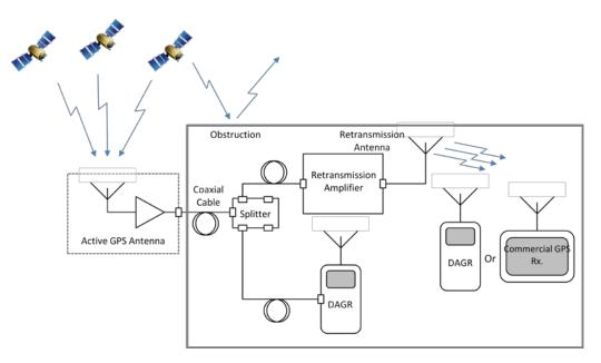
Figure 2. Basic GPS Retransmission System w/ Integrated RF Splitter to Expand System Capabilities
