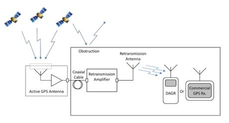
Figure 1. Basic Components of a GPS Retransmission System in US Military Aircraft
