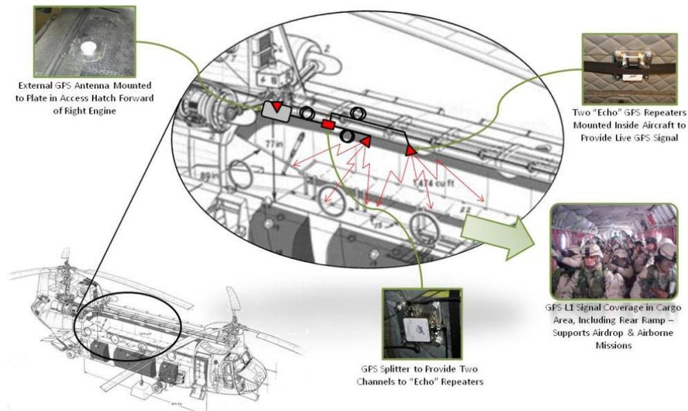
Figure 6. GPS Retransmission System Aboard US Army CH-47
