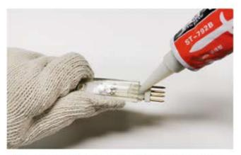
3). Seal the vacant space in the PVC strip at two ends with glue. The glue can't cover to LED. It is better to wait 3-5min until the glue dry. Please notice the has +/- difference.
