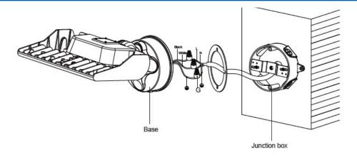
1. Take out the lamp, disconnect the power supply, pass the power cord through the junction box and fix the junction box on the wall. Fix the lamp power cord through the base and fix it with a nut. Put the black wire, white wire and yellow rolling green wire passing the gasket respectively and
