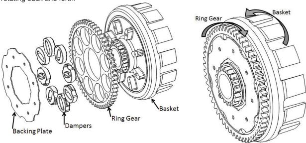
Rotate basket and ring gear in opposite directions to check for any rotational play in the dampers
