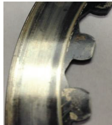
Excessive Heat (Black)
