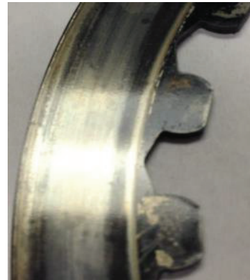
Excessive Heat (Black)
