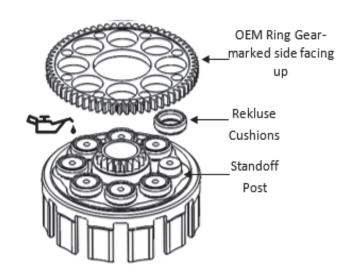
**NOTE:** KX250F baskets have a Bellville spring washer between the ring gear and backing plate, **DO NOT** re-use this.
