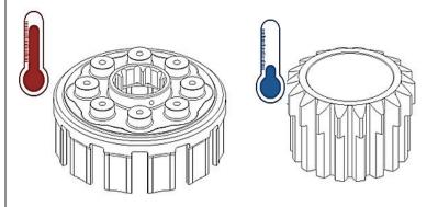
7. After 20 minutes, remove the starter gear from the freezer, then use oven mitts to remove the basket from the oven.
