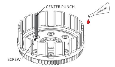
**WARNING**: It is *critical* that you apply Loctite and peen the ends of the screws or they can back out during use. Rekluse is not responsible for engine damage caused by screws that back out.
