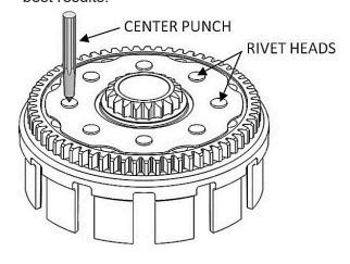
**WARNING:** Drill only deep enough to pop the rivet head off. Do not damage the steel ring gear; it will be reused.
