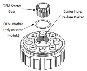
9. If the fit seems too tight, a rubber mallet may be used to tap the gear in while supporting it (such as supporting the basket using a block of wood). Tapping the gear in while the tangs are resting on a hard surface may damage the basket.
