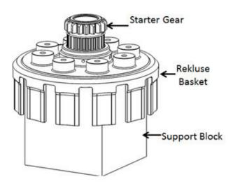
Once the basket has cooled, install the set screw [#47.1]. Use some of the included red Loctite® 262 on the threads of the set screw. Torque to 18 in-lb (2 N-m).
