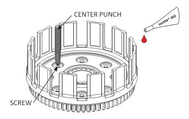
**WARNING**: It is *critical* that you apply Loctite and peen the ends of the screws or they can back out during use. Rekluse is not responsible for engine damage caused by screws that back out.
