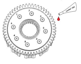
14. Using a hammer and center punch, peen the ends of the screws where they come through the bottom-inside of the clutch basket. Be sure to peen the screws. **DO NOT** peen the aluminum basket.
