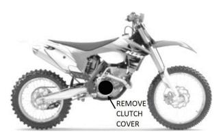
1. Following the procedures in your OEM service manual, remove the existing clutch basket from the engine.
