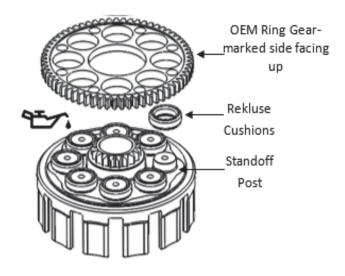
**NOTE:** KX250F baskets have a Bellville spring washer between the ring gear and backing plate, **DO NOT** re-use this.
