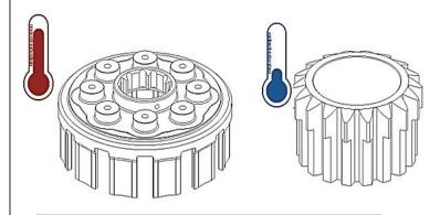
7. After 20 minutes, remove the starter gear from the freezer, then use oven mitts to remove the basket from the oven.
