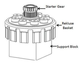
10. Once the basket has cooled, install the set screw [#47.1]. Use some of the included red Loctite® 262 on the threads of the set screw. Torque to **18 in-lb** (2 N-m).
