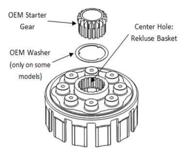
9. If the fit seems too tight, a rubber mallet may be used to tap the gear in while supporting it (such as supporting the basket using a block of wood). Tapping the gear in while the tangs are resting on a hard surface may damage the basket.
