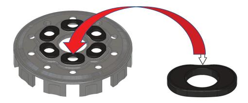
**Note:** The dampers are directional. Place the concave portion of the damper towards the inner diameter of the basket.
