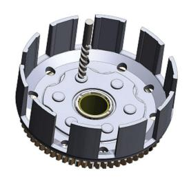
1. Separate the gear from the basket, the gear will be reused.
