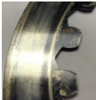
Excessive Heat (Black)
