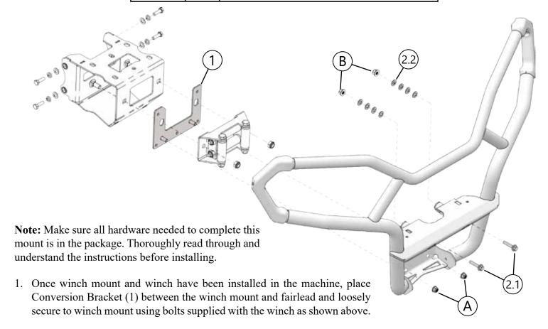
2. Set bottom of front bumper over the studs on Conversion Bracket (1) and secure using OEM nuts (A). Secure top of the front bumper using the supplied bolts (2.1), and OEM nuts (B) as shown above. Tighten all hardware evenly.
