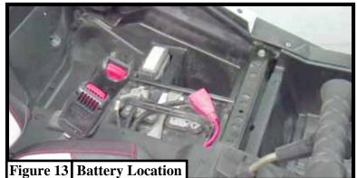
(battery is located under driver seat)
