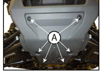
"Figure 2" Plastic Shroud Removal
