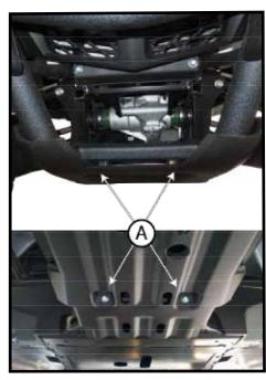
"Figure 2" Plastic Shroud Removal
