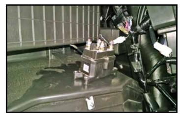
"Figure 11" Contactor Location Passenger Side Inner Wheel Well
