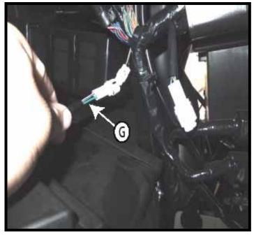
"Figure 14" Wire Location Under Passenger Side Fender
