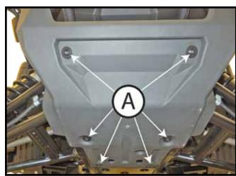
"Figure 2" Plastic Shroud Removal
