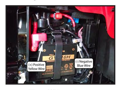
"Figure 10" Battery Location (Battery is located under the rear passenger fender.)
