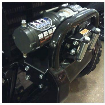
"Figure 8 Winch and Mount Installed"
