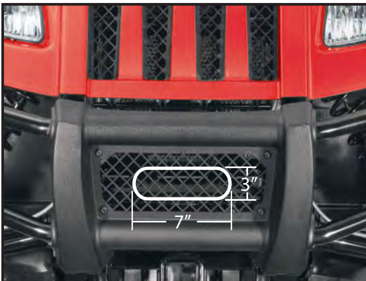
“Figure 3” Trimming Zone
