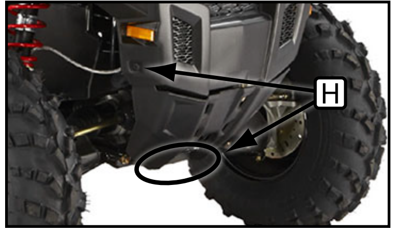
"Figure 10" Lower Front Panel Removal
