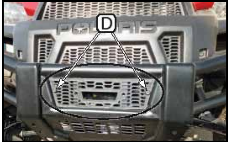
“Figure 4” Bumper Grill Removal
