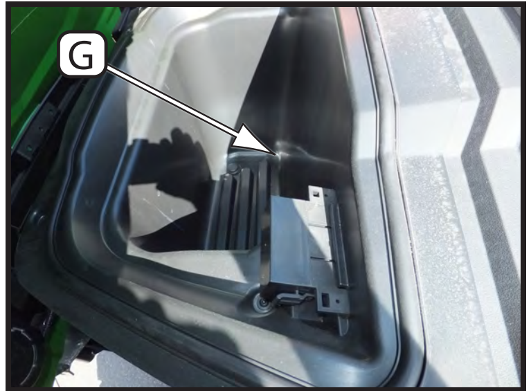
“Figure 8” Contactor Location
