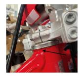
If you have a 3mm or larger gap between the bottom of the stock bearing cap and the top of the weld shown, you will not need to make any modifications to the mount or the weld. If the gap is under 3mm modifications may be needed to the clamps or to the weld.
