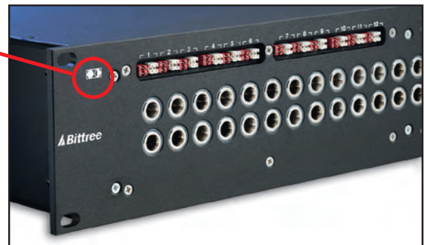
489-S Series Programmable patchbay shown with designation strips removed, exposing red and white external programming shunts on the top row.
