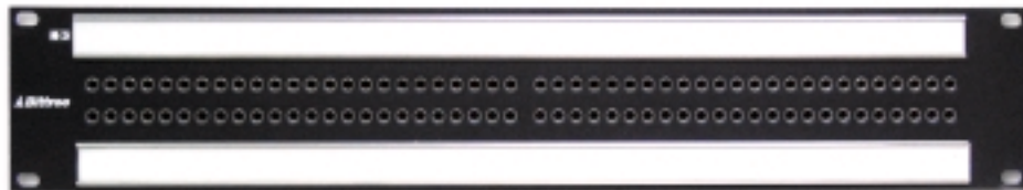
BLACK 2x48 2RU MONO SPACING OVER/UNDER DESIGNATION
