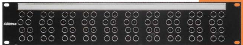
Special RGB-S video patchbay shown with a single row of 20 grouped signal paths. The grouped RGB signals are patched with an RGB patchcord while the S signal is patched via a standard video patchcord
