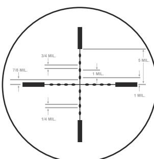
1 mil (millirad) equals 3.6 inches at 100 yards or 36 inches at 1,000 yards, or 10 centimeters at 100 meters or 1 meter at 1,000 meters.
