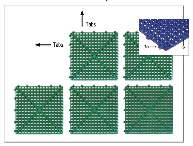
Size up the area you wish to cover. Layout the Dri-Dek Tiles<sup>®</sup> in the desired configuration. Point the outer tabs of the Tiles in the same direction. Dri-Dek Sheets<sup>®</sup> and Rolls<sup>®</sup> will interlock in an identical manner. For large areas, install in independent sections approximately 10' x 10' to allow for ease of cleaning, maintenance and normal expansion and contraction from temperature variations.
