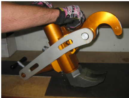
Bead Breaker with pin in highest position
