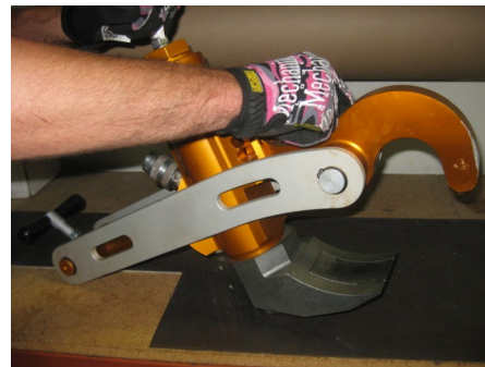
Bead Breaker with pin in lowest position
