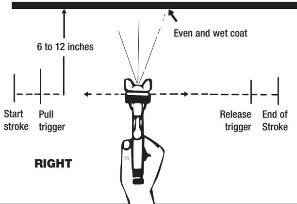
on material and atomizing pressure. For a uniform finish, lap each stroke over the preceding stroke, making sure the spray is smooth and wet.
