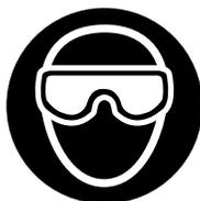
• Always wear impact-resistant eye protection when operating or performing maintenance on this tool.
