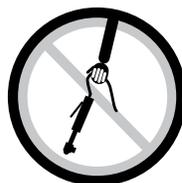
• Do not carry tool by the hose. Protect the hose from sharp objects and heat.
