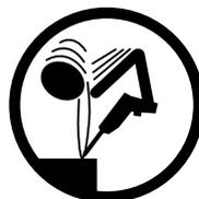
• Keep away from rotating end of tool. Do not wear jewelry or loose clothing. Secure long hair. Scalping can occur if hair is not kept away from tool and accessories. Choking can occur if neckwear is not kept away from tool and accessories.
