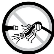
• Air under pressure can cause severe injury. Never direct air at yourself or others. Always turn off the air supply, drain hose of air pressure and detach tool from air supply before installing, removing or adjusting any accessory on this tool, or before performing any maintenance on this tool. Failure to do so could result in injury.
