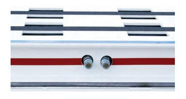
Quick connect no-drip hydraulic couplers, four each side, eight total.
