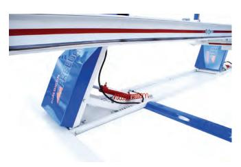
Working height, 14 in. up to 41 in.. Lowers to a loading height of 12 in.
