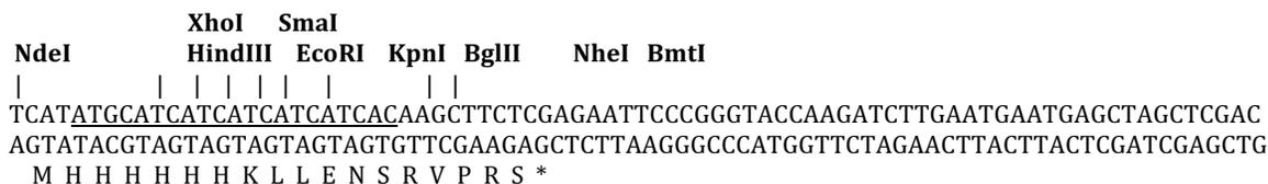
**Figure 1.** Scheme of the vector’s features and map of the MCS. Start codon and sequence encoding 6XHis are underlined.
