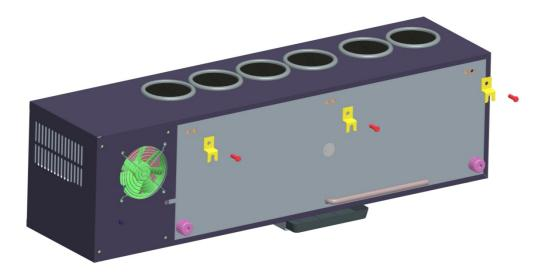
Attach Part A to the back of the unit. Slide Part A into the boring crowns to affix your unit to the wall.
