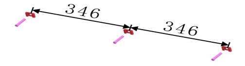
Place the M8 boring crowns against the wall and use them as a guide for where to drill your holes. The diagram above shows the required space between each hole. Use the screws (part B) to affix the boring crowns to the wall.
