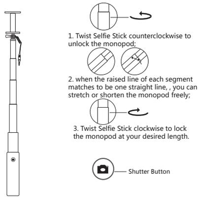
1. Twist Selfie Stick counterclockwise to unlock the monopod;
