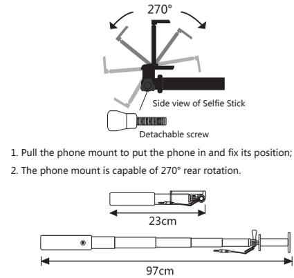
1. Pull the phone mount to put the phone in and fix its position;
