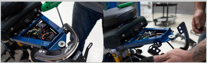
Step 2: Place the included seat spacers on base plate attachment area. Reattach light strip, and secure with BMW bolts. Attach rear seat and you are finished!
