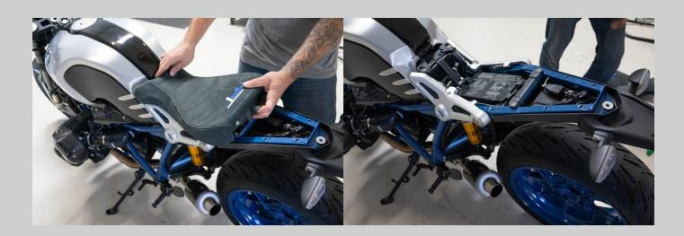
Step 4: Lift up ECU cover and lift ECU. 2017+ models don't require this step, there's no ECU here.
