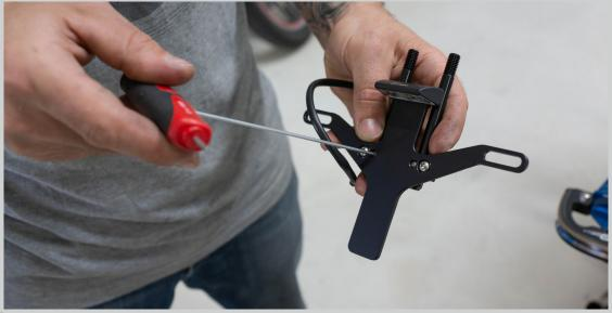
Step 2: Using a T27 Torx wrench and thread-locker (very important), insert light posts into the threaded holes on the underside of the tidy and tighten all the way.
