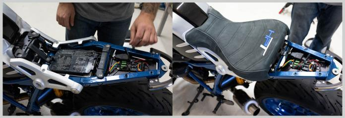
If you're utilizing an integrated light strip and rear cowl, re-install the cowl and you're finished. If choosing to use a rear seat or external signals, continue on to the subsequent installation guides.
