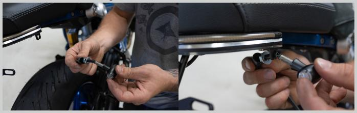
Step 2: Angle them parallel to the ground, and tighten with a 12mm wrench.
