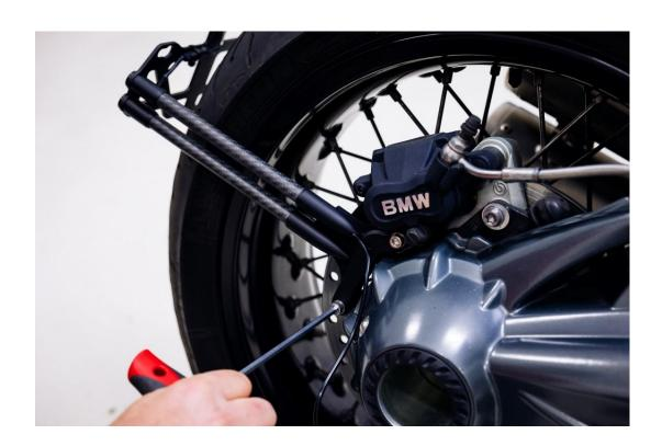
4. Route the harness along the swing arm towards the brake reservoir. We found it best to use one of the supplied zip ties to tie the line to the support beam and tuck the wire in along with the brake line down the side of the arm.
