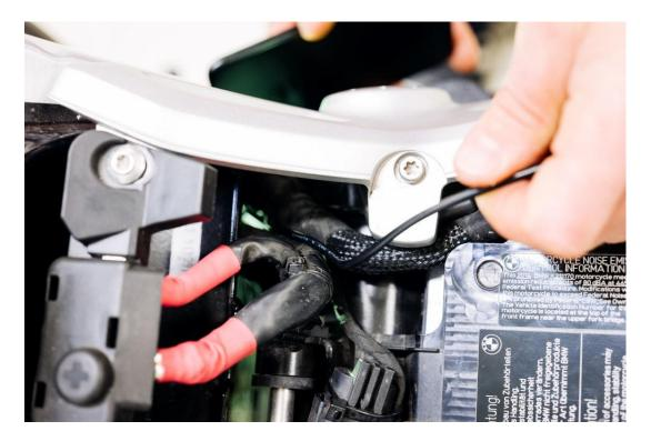
8. Run the wire along the side of the ECU and connect to either our tail tidy harness (shown) or to the tail tidy of your choosing. You can see the swing arm wire running along the top of the photo, above the ECU.
