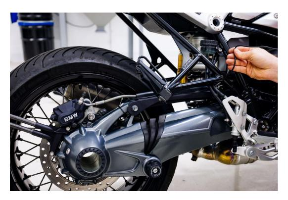
5. Remove the rear seat or rear cowl using the T30 Torx Driver
