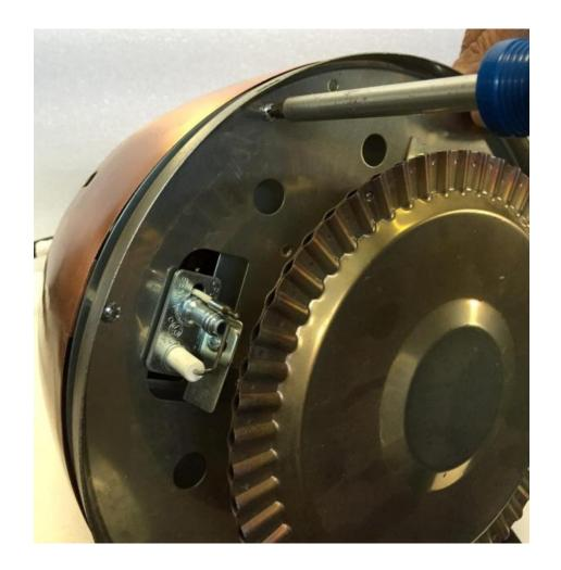
Remove the 8 screws that secure the burner plate to the head assembly.
