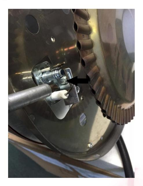
Remove the screw holding the pilot assembly bracket into place.
