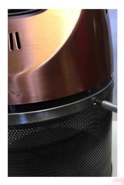
Remove the 4 screws that secure the emitter screen to the head assembly.
