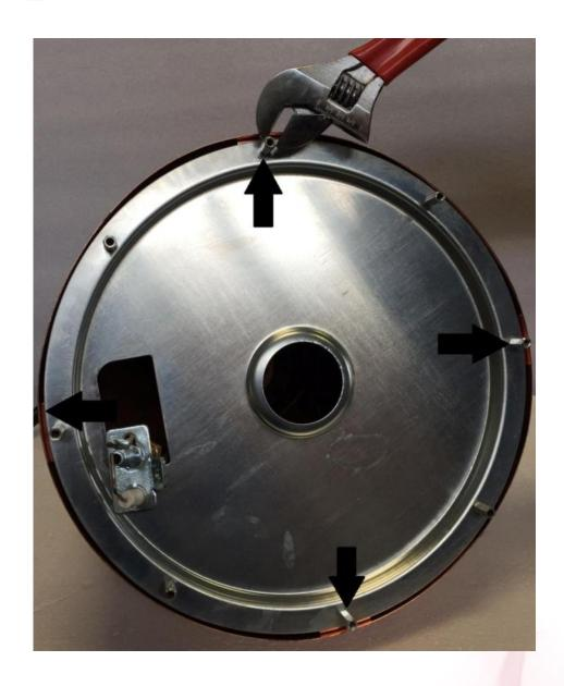
Remove 4 threaded spacers that secure the heat shield in place.
