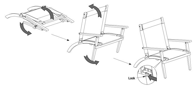
When not in use, the chair may be folded for compact storage. Undo the slide-bolt latches on each side, then fold as shown, being careful not to pinch your fingers.
