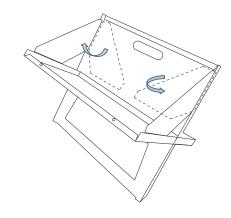
Remove and discard all paper, cardboard, and plastic packaging. Unhook the large cooking grate from the exterior of the grill and set aside.
