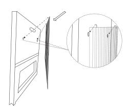
Place the smaller grate inside the grill, supported by the metal lip on either end of the grill. This is the surface upon which you will light your fuel.
